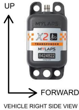
Figure B-57: Transponder Orientation
