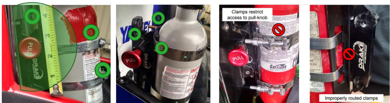
Figure B-45 (B): Fire Extinguisher Mounting, Do’s & Don’t’s
